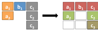
Figure 2: Different algorithms may return different numbers of rows for a given input row. Here algorithms a , b , and c produce 2, 1, and 3 outputs respectively. They are stitched together to create output rows 1, 2, and 3.
